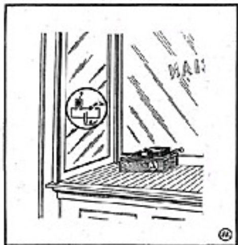
Window Tapper Made From Ordinary Bell and Battery.
